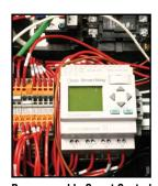
**Programmable Smart Control** Automation provides complete control over the machine's run time, auto start/stop and time delay shutdown functionality.
